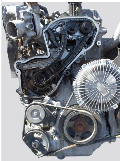
YD25 engine & exposed cam chain
